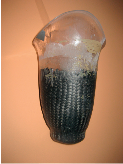
Figure 2.1 A transparent diagnostic socket, reinforced using preimpregnated carbon fiber. Although this is not structurally a desirable solution, it may be clinically necessary.
