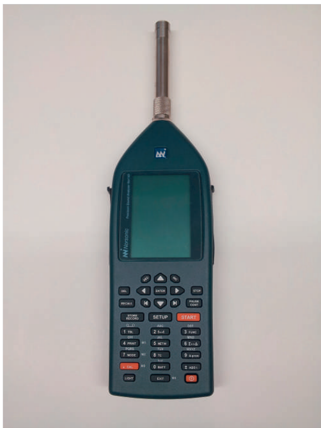
Fig. 1.21 An example of a digital sound level meter with a measuring microphone attached.
